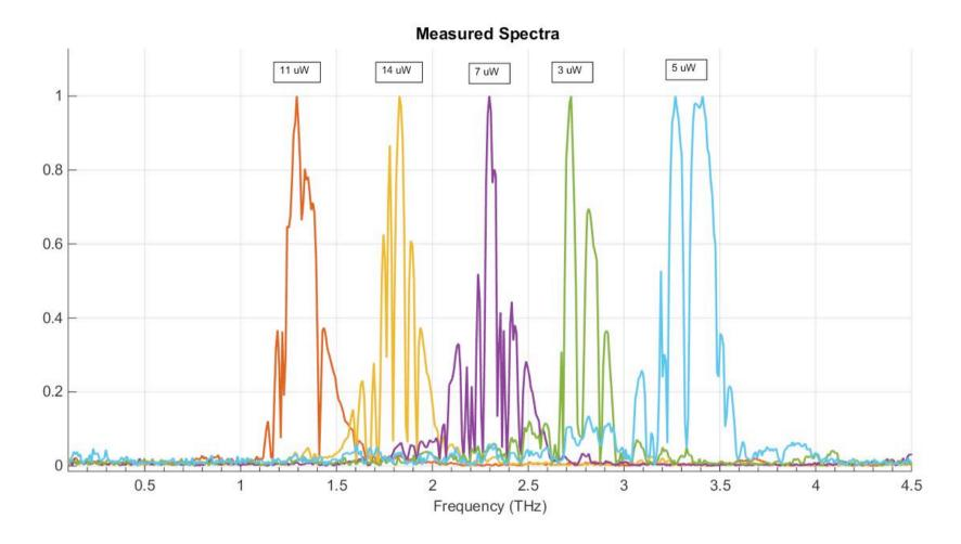
Pulse Duration (inferred from the bandwidth of the pulses): 1-3 ps
